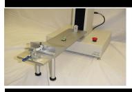
Meets ASTM D-5458 Peel Cling of Stretch Wrap Film Inclined Plane Fixture and COF Carrier Sled w/Pulley Sample Clamp, Wire Stabilizing Legs Included Requires Crosshead Speed of 5.0 ipm
