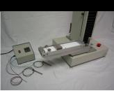
Submersible Tray for Securing Tube Samples Machined Water Bath Pan Temperature Control Console for Water Bath Heaters 70° - 110°F Temperature Range Ports (2) for Addition of Water Recirculation System Requires Crosshead Speed of 6.0 ipm
