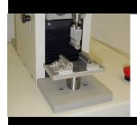
Meets ASTM F-1575 Determining Bending Moment of Nails 3-Point Bending Fixture, Upper & Lower 0.375 inch Cylindrical Bearing Points 1.1 - 2.2 inch Length Between Bearing Points, Adjustable Requires Crosshead Speed of 0.25 ipm
